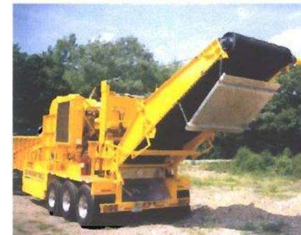
60" discharge conveyor, heavy-duty construction; 15' discharge height; magnetic head pulley available
