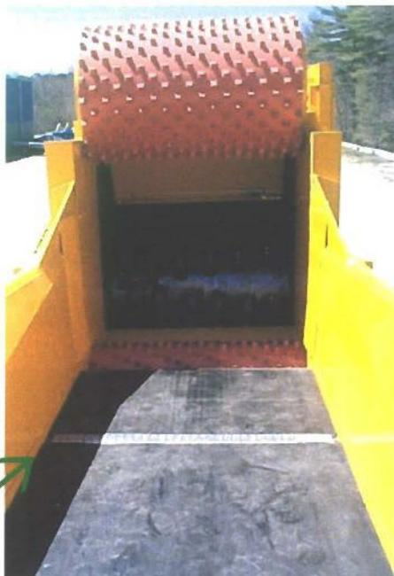
Open ended feed hopper with extra large capacity accepts large surges and full-length material.
