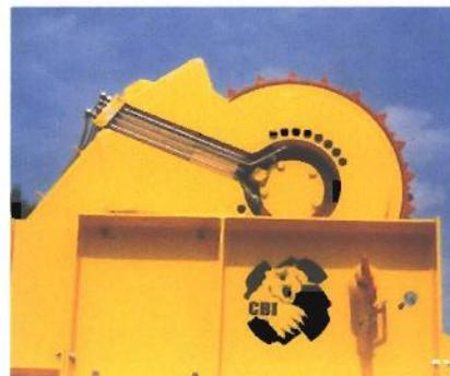
Top feed roller equipped with high-torque internal drive motor.
