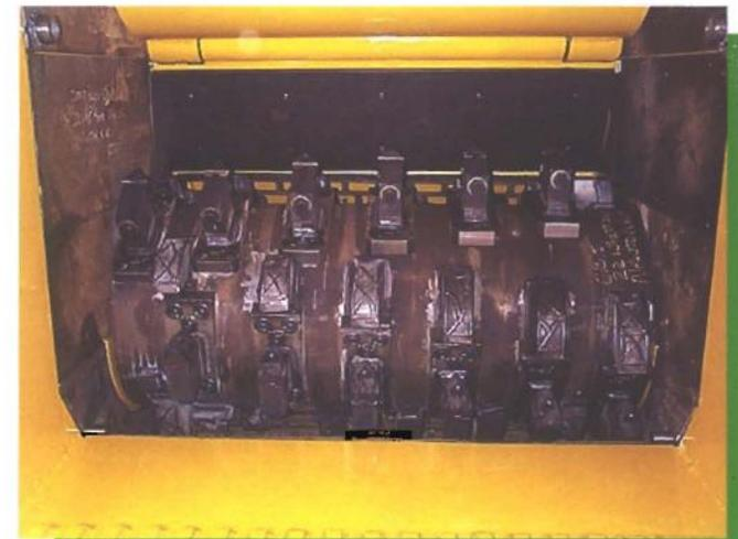
**Unique style hammermill, extreme heavy-duty forged rotor create a patented off-set helix rotor mounted on a 10" shaft, easily replaceable hammer**
